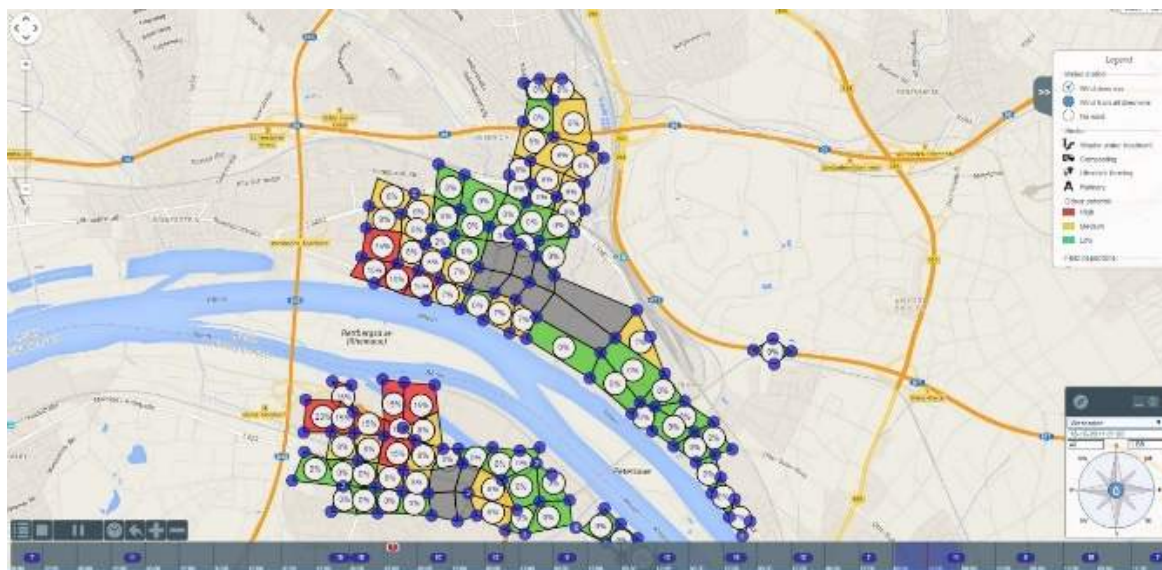
Figure 4: Example of visualisation of field inspection results (Grid Method) in combination with odour observations.
